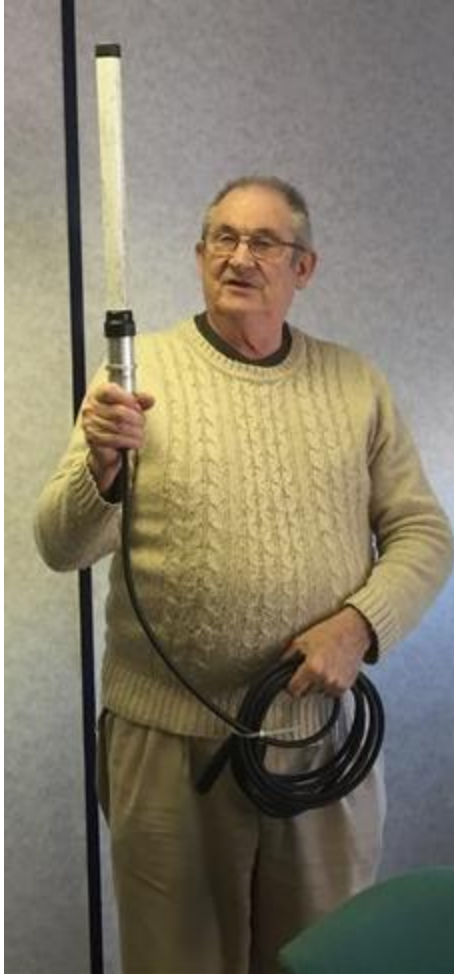
End fed dipole (0dB) ENF450
