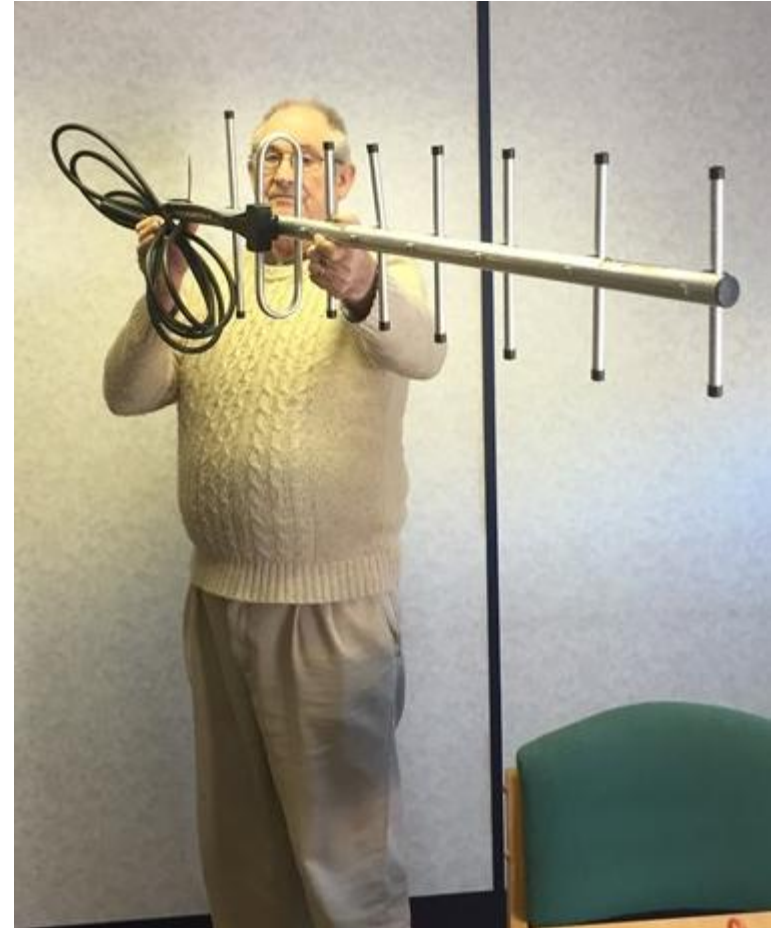
8 element Yagi (10dB) UHF8
