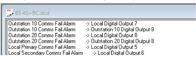
The outstation #10 comms fail alarm is on basestation output 7 and sent to outstation #10 on output 8.
