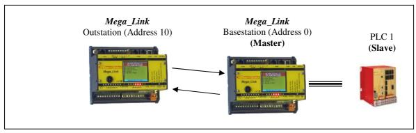
Example 1: Transferring real world inputs & outputs to a PLC slave device via a remote basestation.
