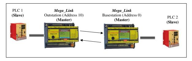
In this example the outstation Data Routing Table would be configured to copy data from PLC 1 to the outstation database, where it will appear as additional I/O. The base-station Data Routing Table can then be configured to pass the outstation's I/O to/from PLC 2.
