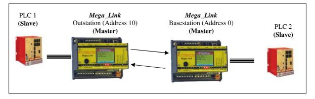
All *Mega\_Link* XTP transfers are configured in the basestation, so inputs/outputs should be viewed from that end. The basestation reads from local inputs and/or outstation inputs and writes to outputs. The *Fieldbus* configuration then has to follow suit.
