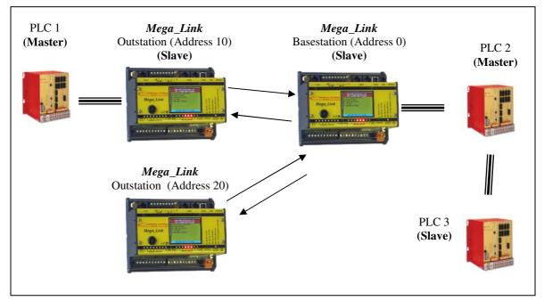
It should be obvious that in this example the basestation and PLC 3 must be configured with different slave addresses.
