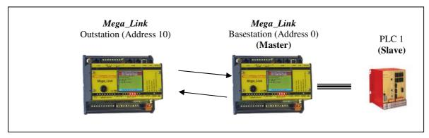
In this example the basestation's Data Routing Table would be configured to pass I/O from the outstation to/from specific registers in PLC 1. PLC 1 will have a defined address that must be used within the basestation Data Routing Table to identify the PLC. It should be apparent that more than one slave PLC could be connected to the *Mega\_Link* basestation, provided the electrical interface supports multi-drop usage.
