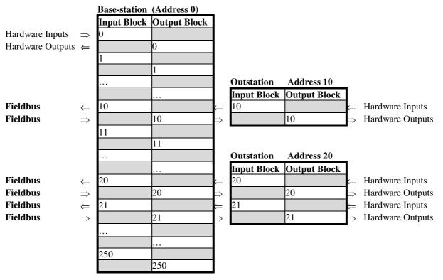
The PLC master will need be configured to identify which data it requires to access, using absolute addressing.
