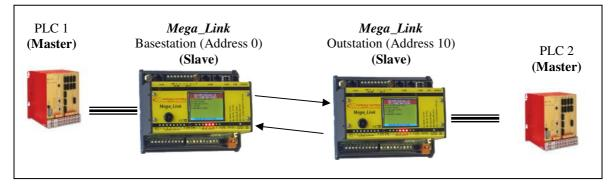
In this example PLC 1 will be configured to copy registers to/from its own database into the outstation database. Similarly PLC 2 will be configured to copy the same registers from/to its own database. The *Mega\_Link* protocol will automatically ensure that the relevant registers within the outstation and the base-station are kept in step.
