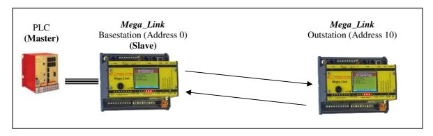
**Example 3:** A PLC master transferring real world inputs & outputs to a remote outstation.
