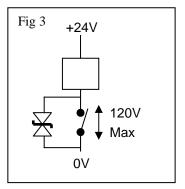
transient suppression diodes fitted across them to clamp the voltage to a maximum of 120V. This limits the maximum voltage that can be switched by the contacts, and also reduces, but does not eliminate, electromagnetic radiation from them.
