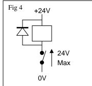
The preferred method of preventing the phenomenon is to fit a diode across each inductive load, as shown in Fig 4. When the switch is closed the diode has no effect, since it is reverse-biased across the 24V supply. When the switch opens the current that was flowing through it flows instead through the diode, hence clamping the voltage across the coil to typically 0.6V. The highest voltage ever present across the open switch contacts is thus equal to the supply voltage.
