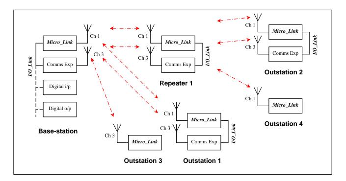
In this illustration the base-station, the repeater and outstations 1 & 2 are equipped with the dual comms facility. It is assumed that all *Micro\_Link*'s except Outstation 3 have radios set to channel 1 and all comms expansion modules, plus Outstation 3, have radios set to channel 3. Note that the scenario could equally be that leased line modems are used in place of radio channel 3, for example.
